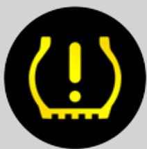
Remember that with every 10 degree drop in temperature, your tire pressure drops one PSI. As most vehicles have mandated tire pressure monitoring systems (TPMS) in place, this means a lot of amber TPMS warning lights will be showing up with winter approaching. If your TPMS light comes on we will be happy to check your tire pressure and re-inflate them back to the proper factory level.
